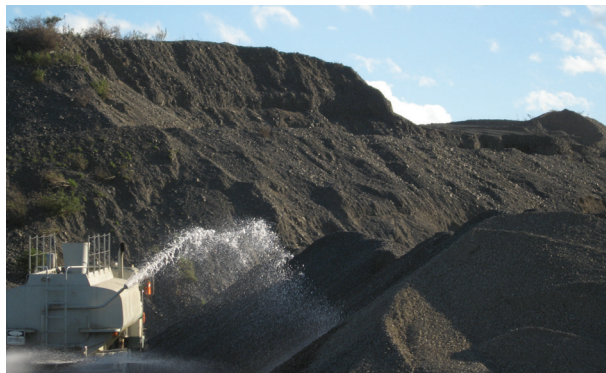
Figure 9 - Controlling dust at stockpiles
