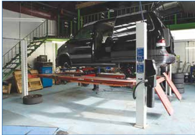
Figure 2.2: Drive-on four-post hoist
